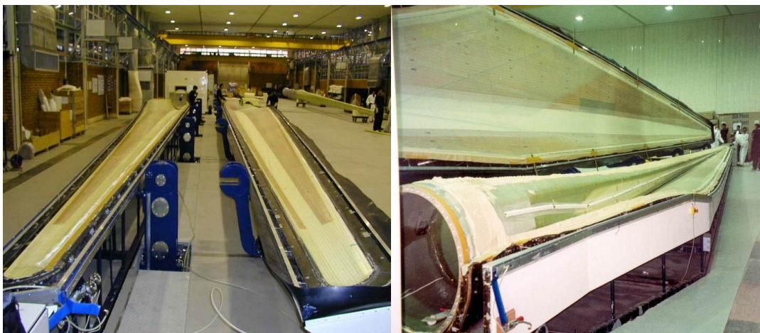
Fig. 1 A production process of a composite wind turbine blade using hand lay-up method (Courtesy of Sabaniroo Co., Iran)
